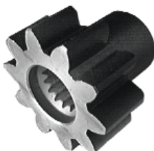
54146-020 Pinion Gear-CW 10T-40.5mm Gear O.D.-40mm L. Replaces Denso: 028099-3270. Used on Drive: 5446-2523
