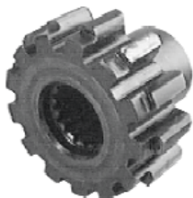
54146-014 Pinion Gear-CW 13T-46.5mm Gear O.D.-36mm L Used on Drive: 5446-3006.
